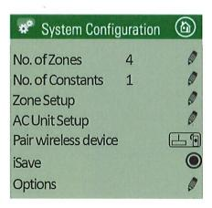
• Pair the WiFi Bridge to the iZone system. Press and hold the blue button on the side of the Bridge. At the same time press the "Pair Wireless Device" button on the touchscreen
